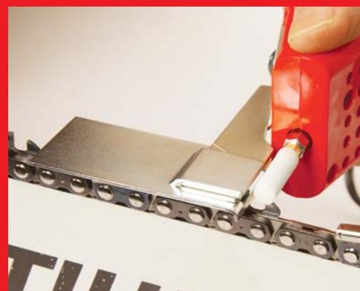
**8. REST GAUGE ON TWO CUTTERS AS SHOWN,** the one to be jointed and the one following. Start grinder and stroke back and forth gently to lower depth gauge to desired height. Lower all depth gauges from the same side of bar as shown.
