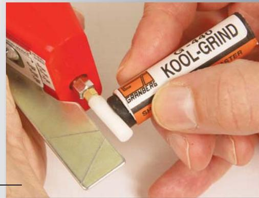
**6. FOR COOLER GRINDING USE 'KOOL GRIND' LIBERALLY.** Generates less heat- stone clogging - extends stone and chain life. To use touch stick to rotating stone after every 3 or 4 cutters sharpened. Ask your dealer for G440 Kool Grind.
