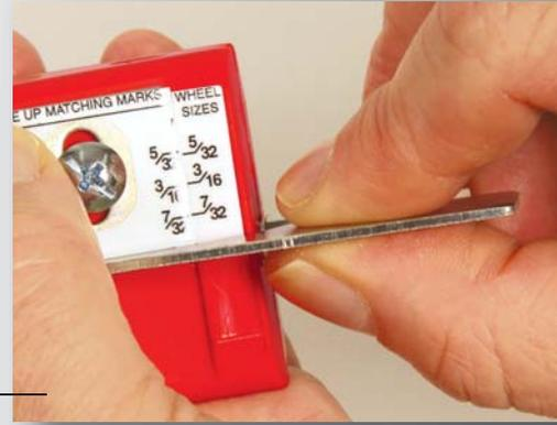
**2. LOOSEN SCREW ON HEIGHT PLATE FOR ADJUSTMENT.** Example: if 3/16 grinding wheel is used, then line up matching marks at 3/16 on wheel sizes gauge and tighten screw.
