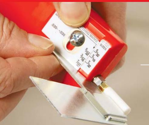
**7. INSERT 1/4" STONE PROVIDED WITH GRINDER** into mandrel finger tight. Also insert #493 depth gauge into height plate as shown. Loosen height plate screw and set height plate scale to desired height. Line up marks and tighten screw. See example .030 aligns with .030
